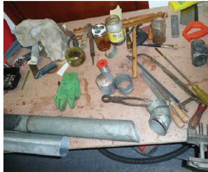
Metal trunks are made up in the time-honoured way with a hot iron, solder, and a hacksaw
