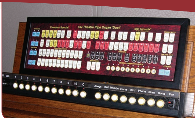
One registers and saves the organ's 208 voices, couplers and tremis to pistons through unique divisional/select system.
