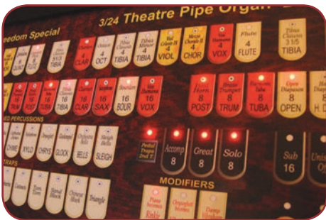
Each stop toggles lightly when touched, and has an LED indicator that glows, showing the stop is "on".
