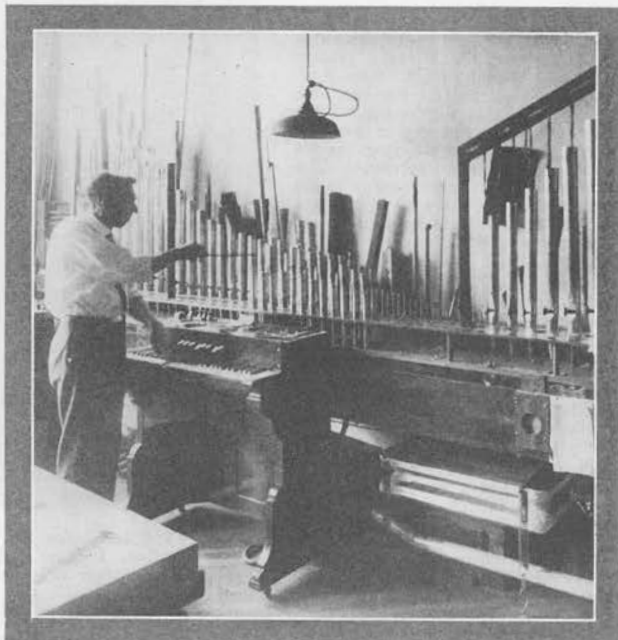
The plate on this page shows a typical installation of a theatre organ at the sides of the proscenium arch. These two scenes are also in the Wurlitzer factory. At left is shown the making of wood pipes, and, at right, the voicing of Vox Humana stops.
