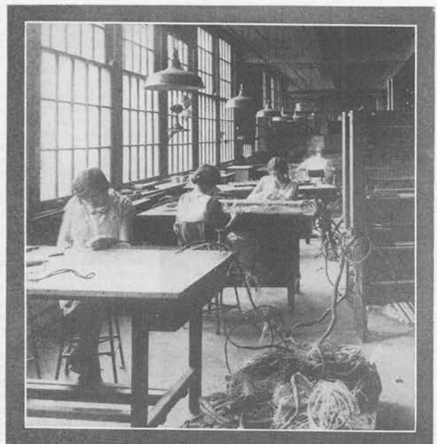
Installing and making an organ. The plate at the top shows a typical installation of an organ chamber above and in the center of the proscenium arch. Below are scenes in the Wurlitzer organ factory, in the magnet winding department (left) and the wiring department.
