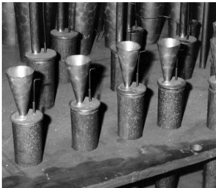
An early Wurlitzer Kinura with spotted metal resonators (Photo by Jim Stettner)
