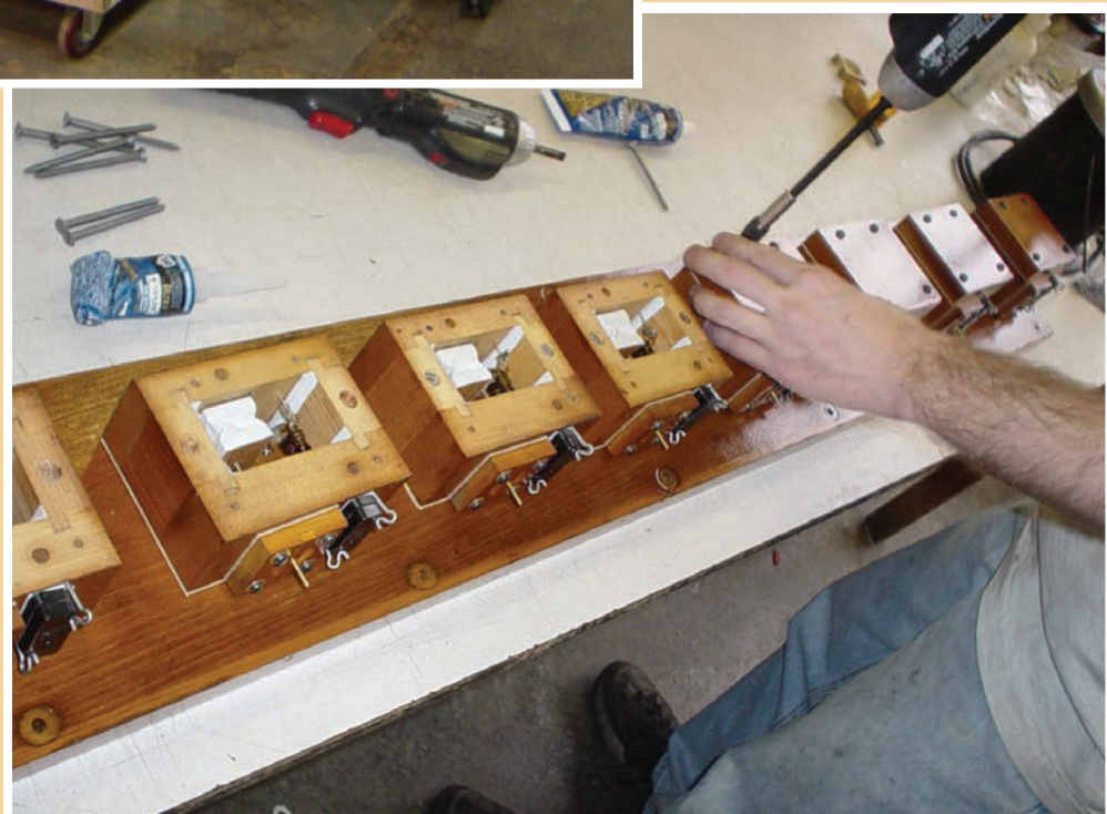
Restored primary boxes
