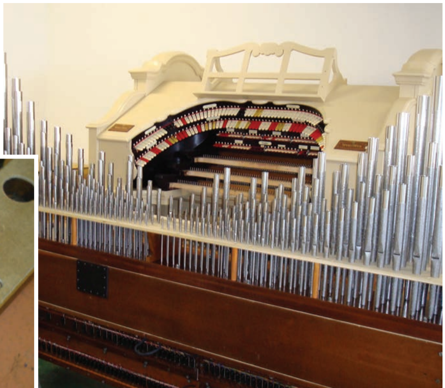
Mixture racked on new toeboard
