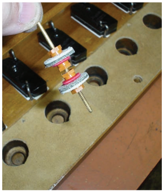
New primary valves
