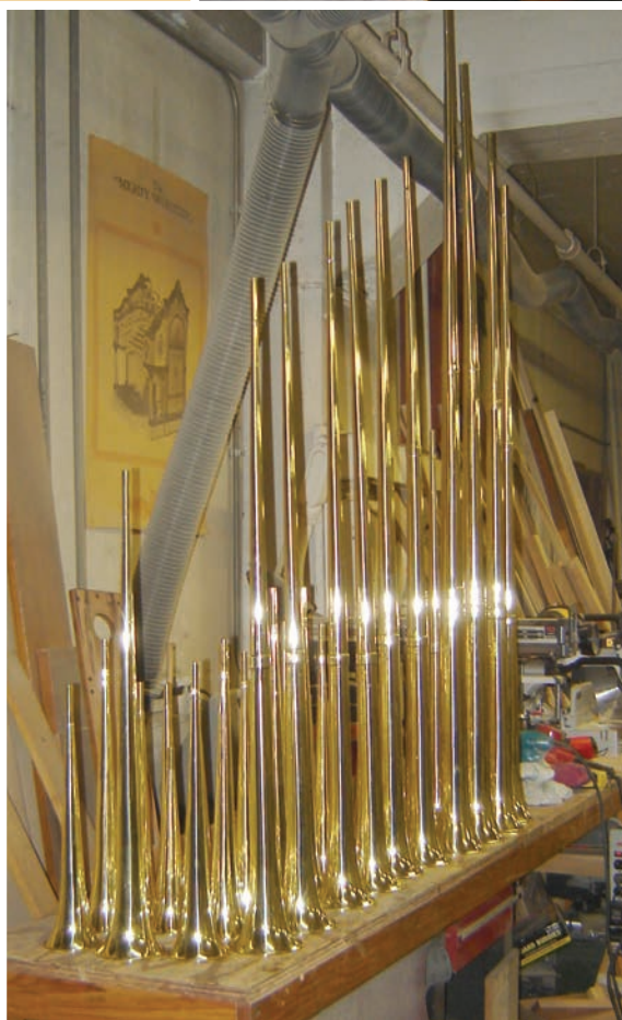
Trumpet resonators after polishing
