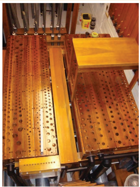
Solo chests ready to receive pipework
