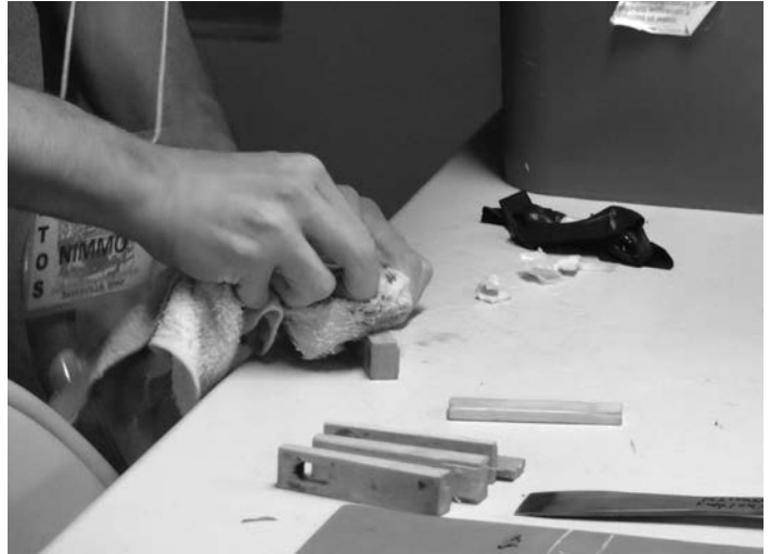
Justin Nimmo uses hot water to carefully remove adhesive residue
