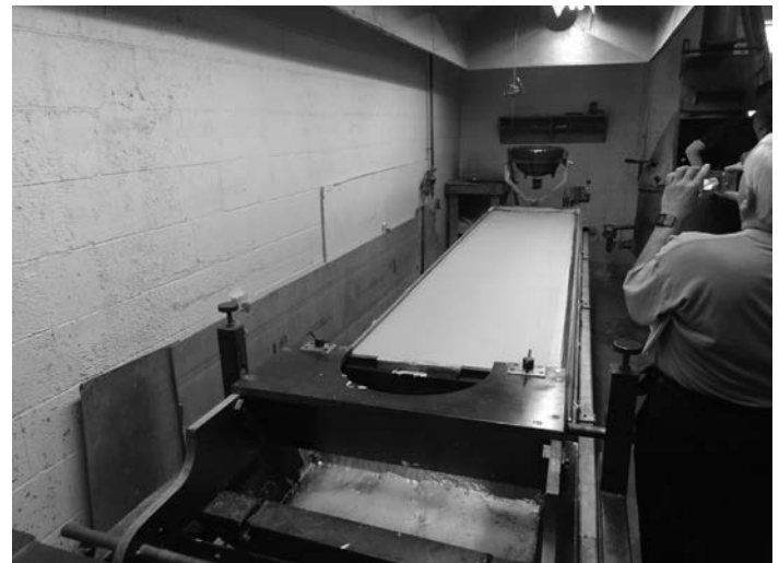
A sheet of pipe metal just cast and cooling. Melting and pouring pots in background, sluice box in foreground.
