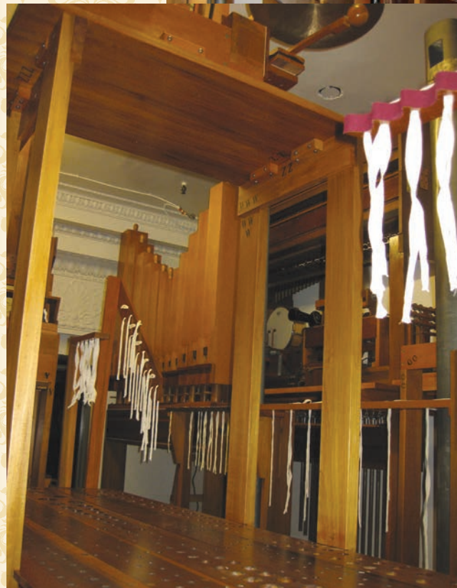
A view of the assembled chamber from the opposite corner next to the main swell shades, main chest in the foreground. The Tibia Clausa offset is behind, and the toy counter and percussions behind that. Directly above the main are the Bass Drum and Crash Cymbal (Jim Stemke)
