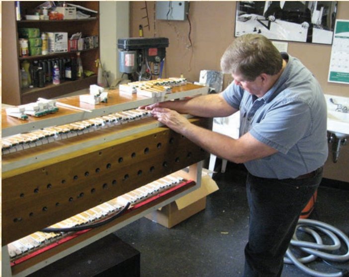
Jim Stemke glues restored pneumatics in the Solo chest (Jim Stemke)
