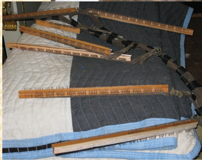
A close-up of the new spreader strips for the console cable showing the original cotton covered cable (Jim Stemke)
