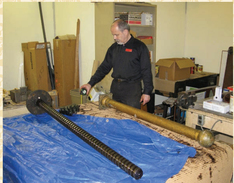
Curator of Organs Curt Mangel with one of the four posts from the Barton lift. The gold decorative cast-iron housing covers the large screw (Jim Stemke)
