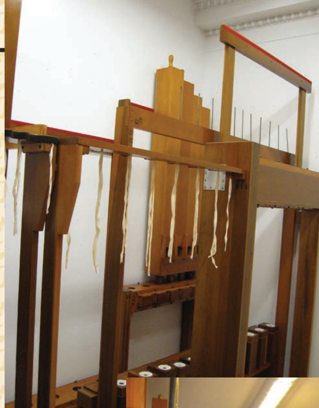
More offset chests are assembled and restored Bourdon pipes test fit in their chest (Jim Stemke)
