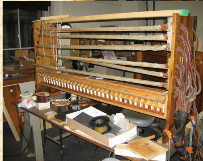
The relay completely dismantled in the shop for restoration (Jim Stemke)
