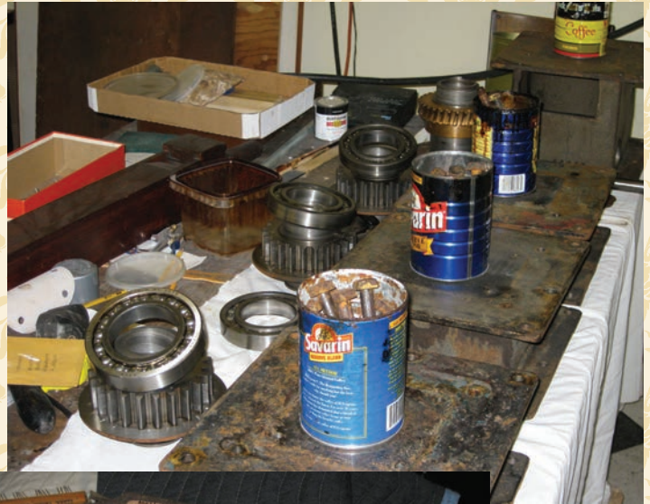
Disassembled parts of the drive mechanism of the Barton Four-Poster Lift for the console (Jim Stemke)
