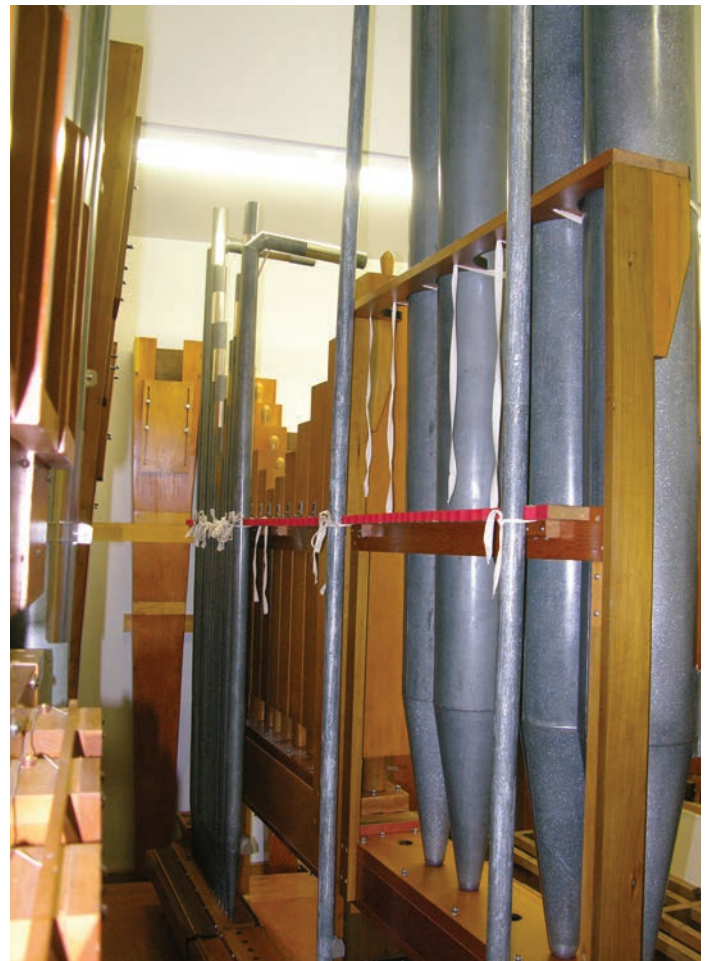
8' String offsets (four ranks) are mounted behind the 8' Tibia and 8' Diaphonic Diapason. The Diapason and Tibia chests are elevated to provide clearance for the mouths of the strings (Photo by Mike Bryant)
