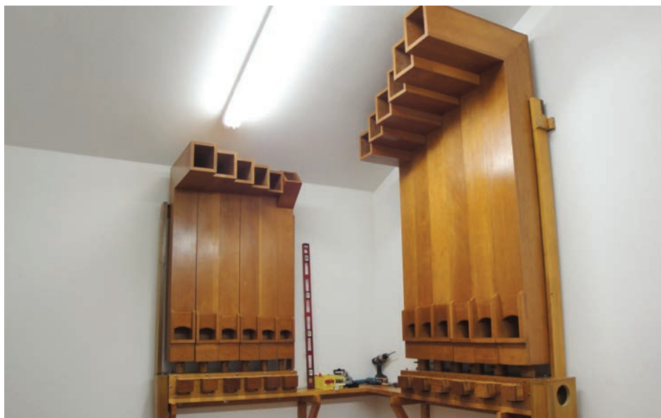
16' Bourdons were mitered to fit. The shelf is part of a water-damaged Robert-Morton Bass Flute. The set was incomplete and beyond repair as a pipe, but after two years of drying, it milled down just fine for this use (Photo by Bob MacNeur)
