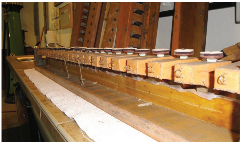
Speaking of "how not to," notice the adhesive mounting the secondaries to the chest. This is sometimes referred to as "organ builder in a tube" and is not generally considered an appropriate adhesive or gasket material (Photo by Bob MacNeur)
