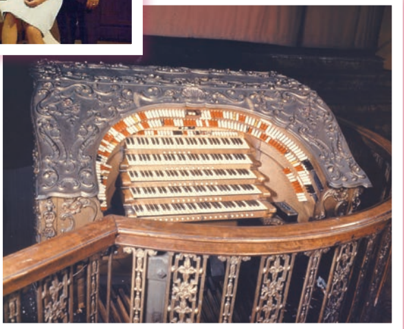
Prior to its removal from the Marbro, the console shows its original finish, as well as evidence of Wurlitzer's modifications in 1930: tape on short key rail stop keys, and a new stop key for Solo to Great Sub (John Shanahan Collection)
