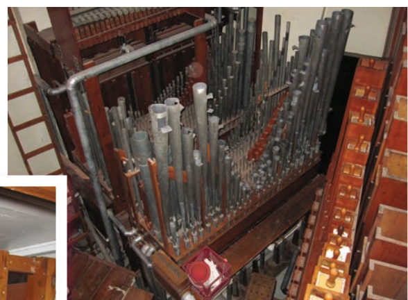
The Main chamber as it looks today. Much of the framing from the Marbro was used, both in the Carlson installation, and in Providence, resulting in chamber layouts that closely resemble the original. The massive wall of swell shades at the Marbro was greatly reduced in Providence, due to significantly smaller chamber openings at PPAC (Jonathan Ortloff Collection)
