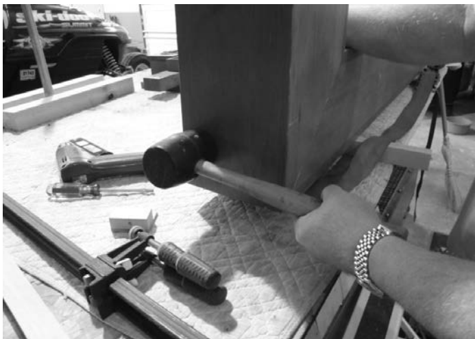
Figure 18. Gently persuade everything into place before applying clamping pressure
