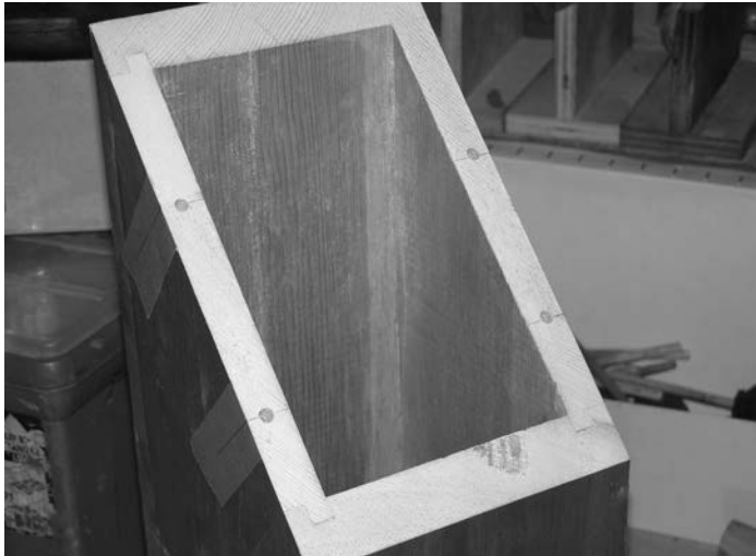
Figure 16. Holes are drilled, ready for dowels and joinery
