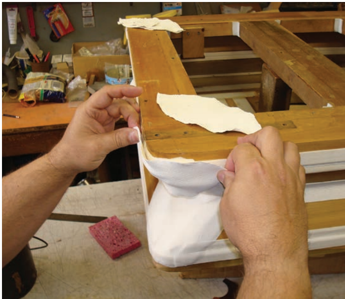
Carlton Smith applies corner patches to a regulator (Photo by Justin Nimmo)
