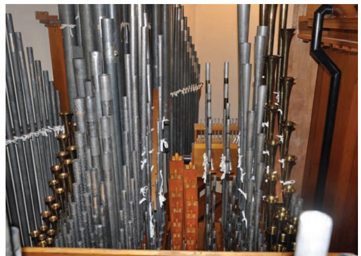
Solo Chamber after reinstallation, L-R: String offset, Saxophone, Quintadena, Horn Diapason, Krumet, Orchestral Oboe, Tibia, Solo String and Celeste, English Horn, Trumpet, Vox Humana (Photo by Matt Madden)
