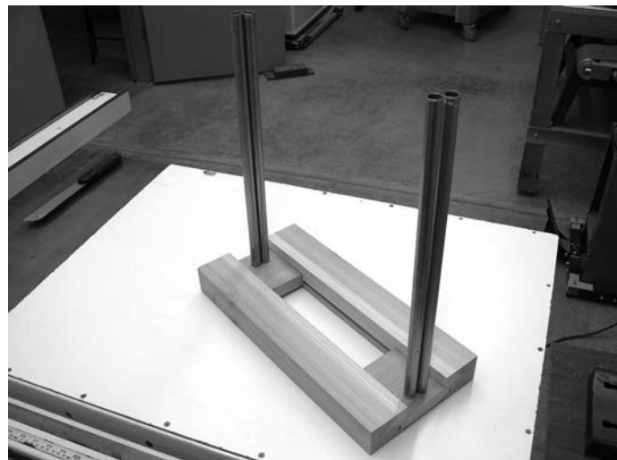
Figure 3. Shop-made miter guide: scrap wood, dowels and 1/2" conduit
