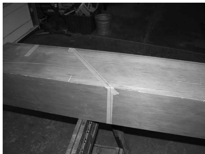
Figure 4. Lay out the cut line on painter's tape
