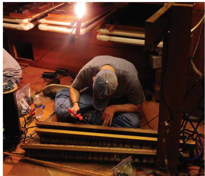
Soldering magnet wires to bottom boards (Photo by Matt Madden)
