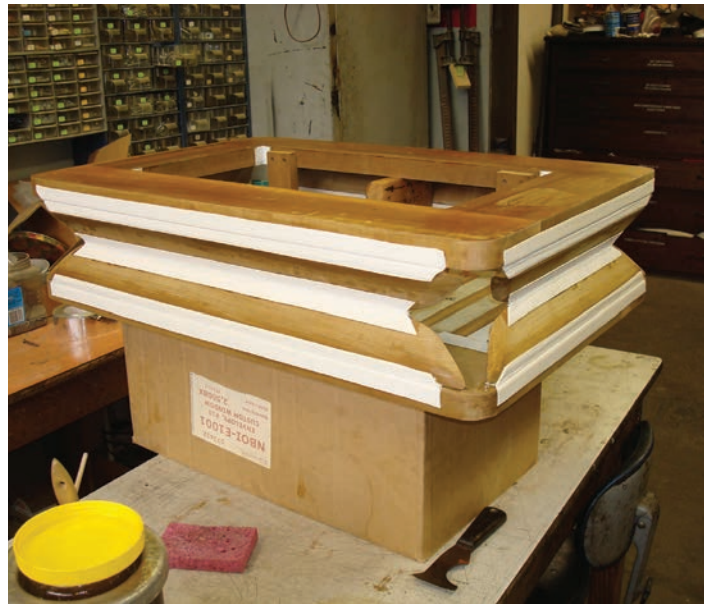
Reservoir all hinged and ready for gussets (Photo by Carlton Smith)
