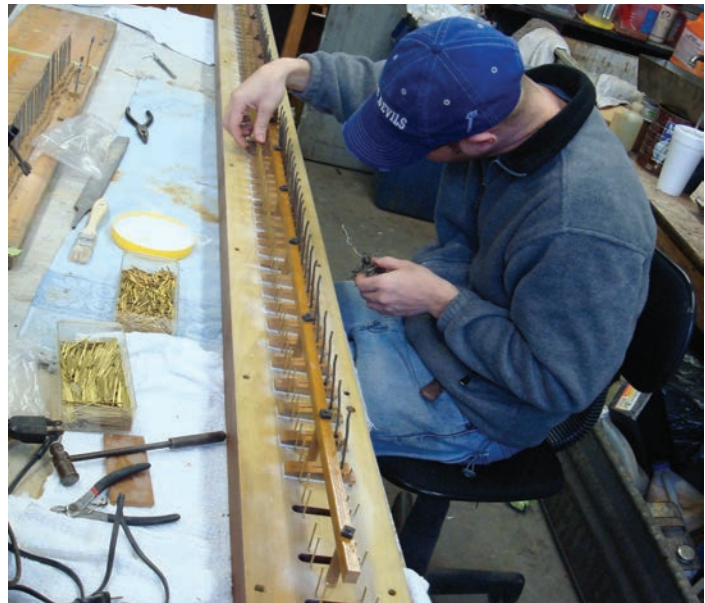
Justin Nimmo assembling pallets on restored toe board (Photo by Carlton Smith)
