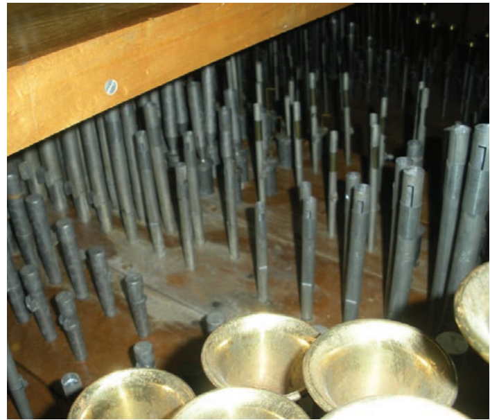
Water damage on rackboards (Photo by Matt Madden)
