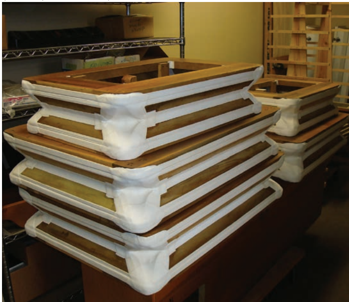
Newly-leathered regulators, ready for installation (Photo by Carlton Smith)
