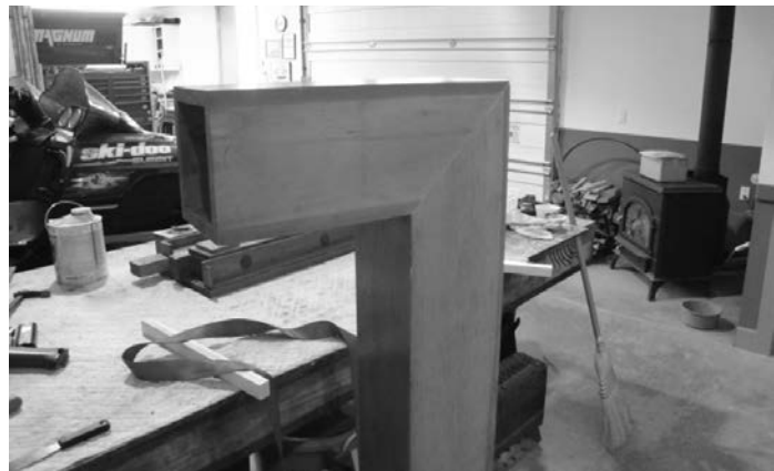
Figure 20. An almost-invisible seam. Touch up with a bit of stain or shellac, and it's ready to install
