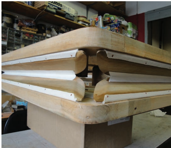
Reservoir rebuild in process (Photo by Justin Nimmo)
