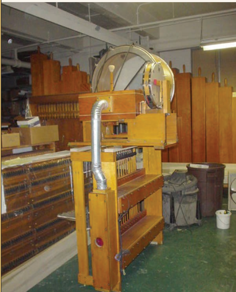
Drum unit mounted atop the Chrysoglott
