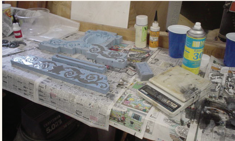
Casting the reproduction console ornamentation
