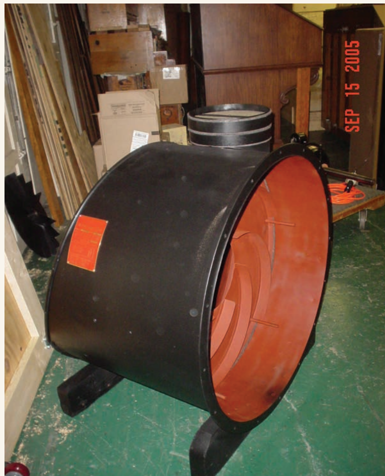
The restored Spencer blower
