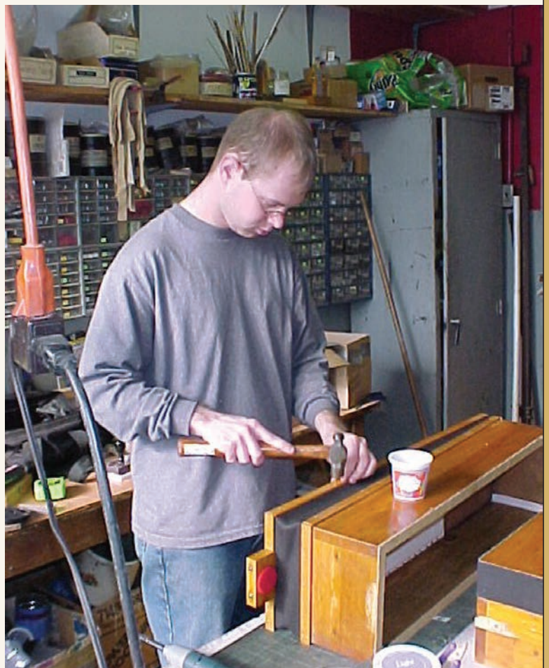
Justin Nimmo works on a tremulant assembly
