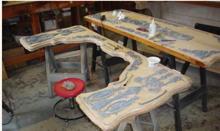
The replica ornamentation is applied to the console panels
