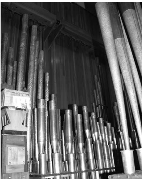
The Wurlitzer Vox Humana, with the Gamba and Celeste behind. The upper shutters are Wicks, the lower set (not visible) is Wurlitzer. All shutters are closed when the organ is off, allowing chamber temperatures to be regulated independent of the sanctuary.
