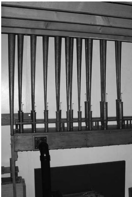
Because only one note of this Möller Tuba is mitered, the chests for the 8' and 16' octaves are mounted below the chamber floor
