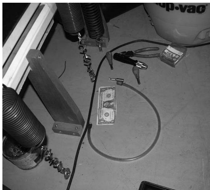
A pin vise, dag tools, clear tubing, and a reed cleaning tool stay in the chamber
