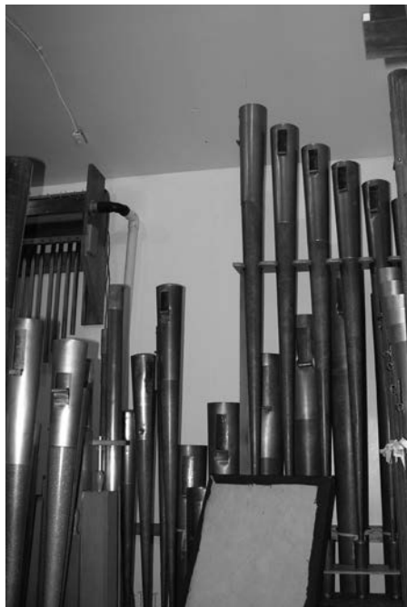
The Möller Tuba resonators can be seen behind the French Horn offset
