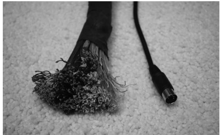
Fig. 3: Organ console cable vs MIDI cable
