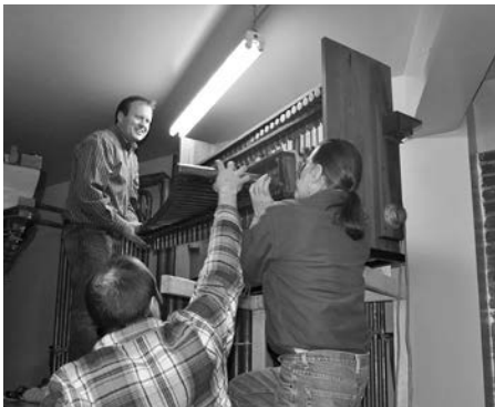
Puget Sound Chapter members (l-r) Tom Blackwell, Jake Cihla, and Phil Hargiss place the Seattle Paramount Wurlitzer Chrysoglott bars back into the action frame (Photo courtesy Tom Blackwell)
