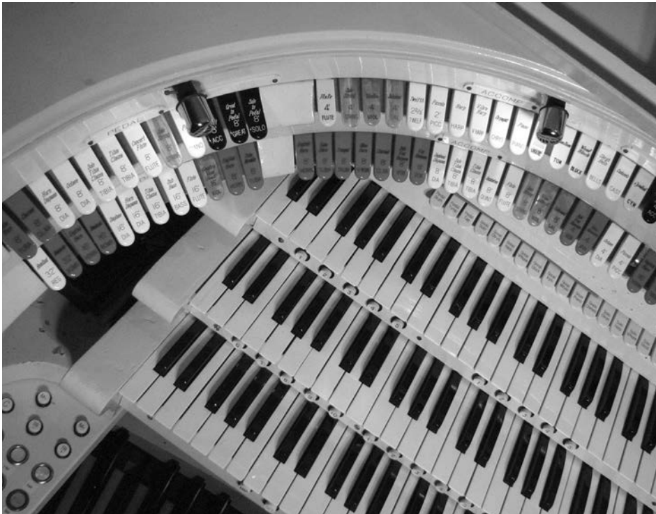
Left: New Syndyne stop switches and tabs were installed to match the current configuration
