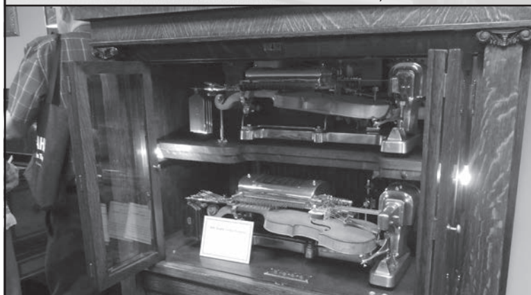
Very rare Mills Double Violano Virtuoso—since each string of each violin is "bowed" independently, it is possible to play up to eight-part harmony on the violins, along with the 44 piano notes
