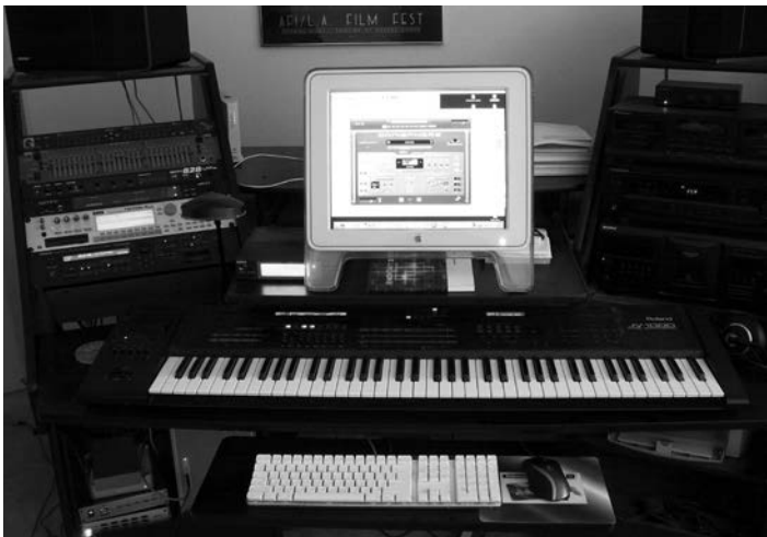
My home rig consisting of keyboard controller and sound hardware. The majority of the resources are in virtual instrument programs and sample files that reside in the computer
