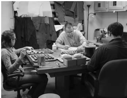
Susan Johnson, John Riester, and Chris Ganza leathering primary pneumatics at the AOI shop
