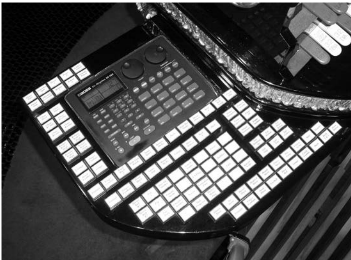
Left drawer incorporating the DR-550 drum machine
