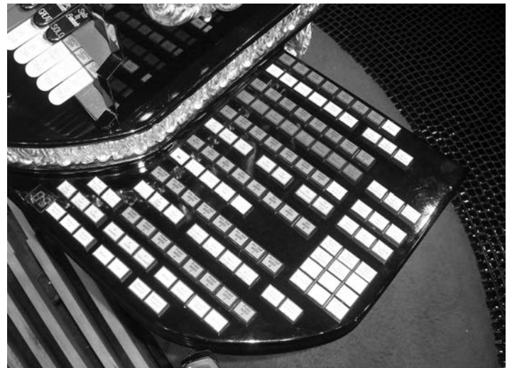
Right drawer with selectable ranks and Midi controls; 8 Midi channels per division including Acc. Second Touch
