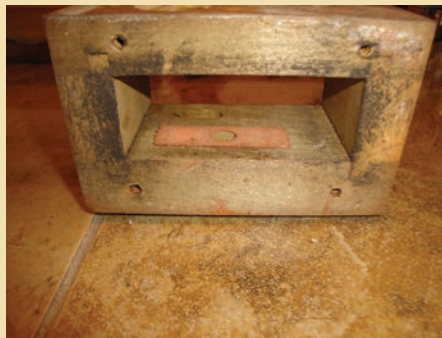
We found a few gaskets covering holes: this was in a primary box...
