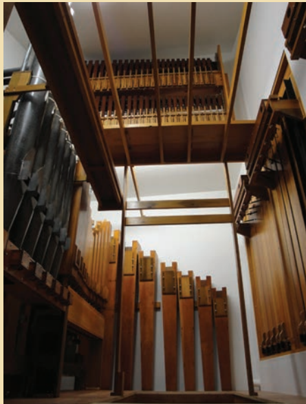
Below the harp, the framing for the upper toy counter is shown
