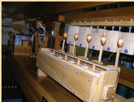
From right to left, the lower toy counter holds a set of Temple Blocks (five blocks), toy counter manifold, Shuffle, Acme Siren, and Arndt double cymbal action
