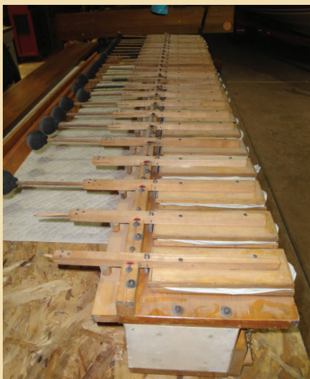
The Morton Harp was missing several mallets and shanks when it was acquired, and a number of arms were badly warped
