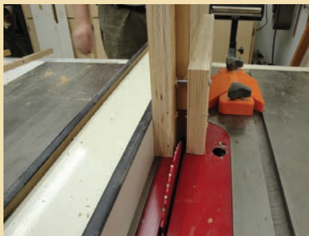
The new arms were mounted in a fixture and run through the table saw with a fine-kerf blade to make the clamping slot
