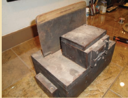
This Wurlitzer Shuffle unit went through a fire and suffered water damage. Although it isn't visible in this shot, the top plate was warped and required replacement
