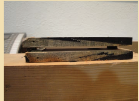
Not only was it off side-to-side, but the fixed and movable halves were different lengths
