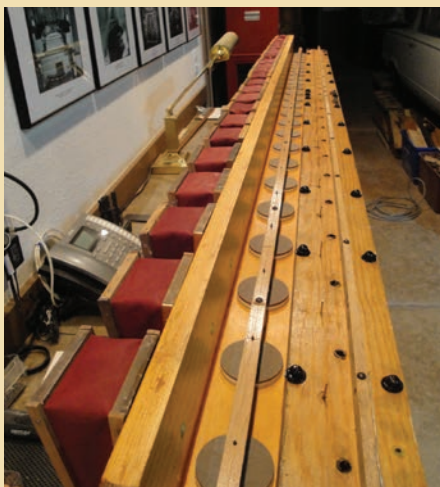
The action is assembled; next step is to mount the arms to the power pneumatics
