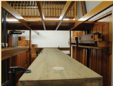
Here, you see the lower toy counter trunk being test-fit
