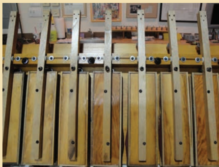
A mix of old and new; can you spot which is which? (The center three arms are new; the others are original)
