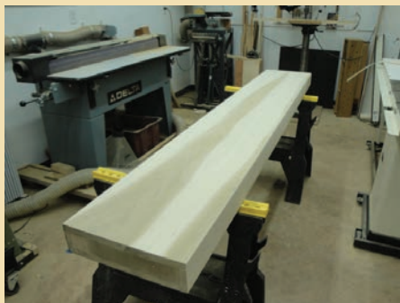
After everything was laid out on a paper template, the newly-plugged trunks received new poplar veneer
