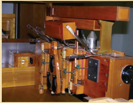
The toy manifold contains the Train Whistle, Bird Whistle, Triangle, Wood Block, Fire Gong, and Castanets
