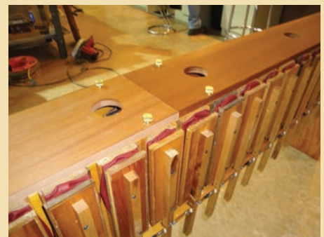
The mufflers have been cut and fit, the inserts for the thumbscrews are installed, and they are ready for finishing. When installed, they make a huge difference in the noise of the action
