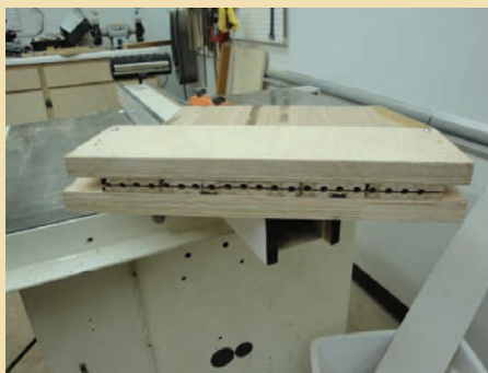
The arms were drilled to accept the shanks before the slot was cut
