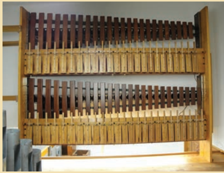
The almost-finished Robert-Morton harp. The mallets will be installed when it's wound
