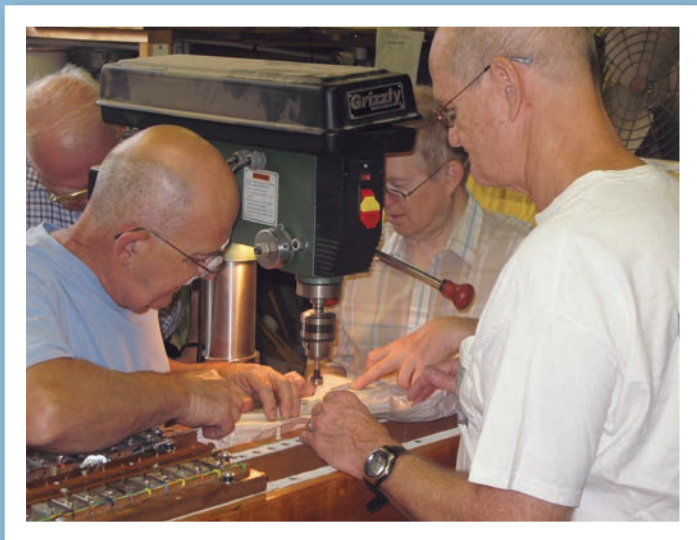
Andy Gallien, Glenn Felten, Tom Cronier, bore out a new hole for the brass insert
