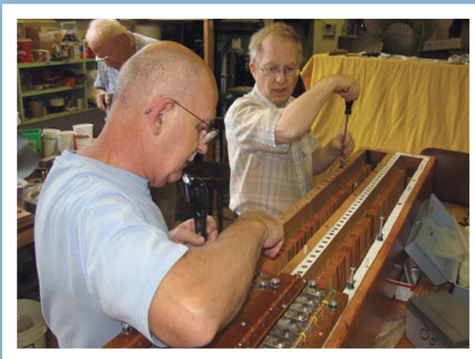
Andy Gallien and Glenn Felten installing brass inserts on the Musette/Violin chest
