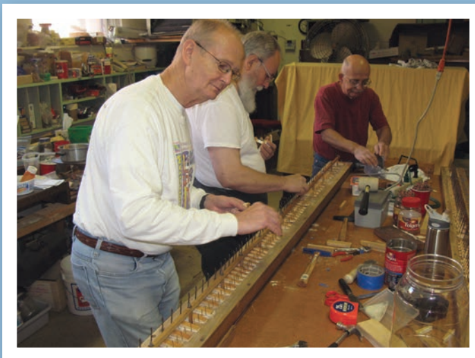
Tom Cronier, Larry Donaldson, and Andy Gallien assemble a toe board
