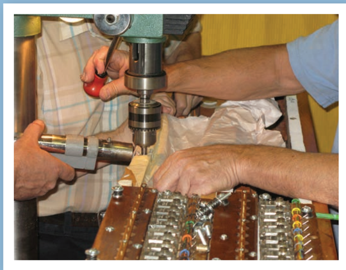
Chest surgery: boring out a new hole for the brass insert
