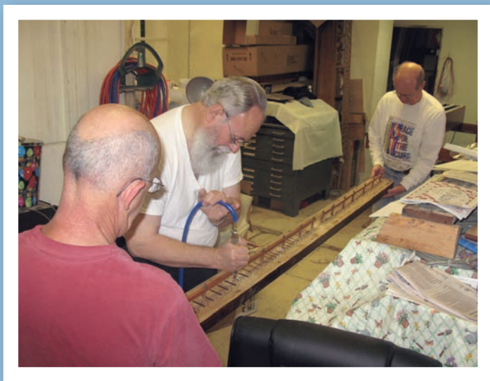
Blowing out the toe board
