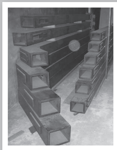
16' Violone in the String chamber; note the horizontal installation
