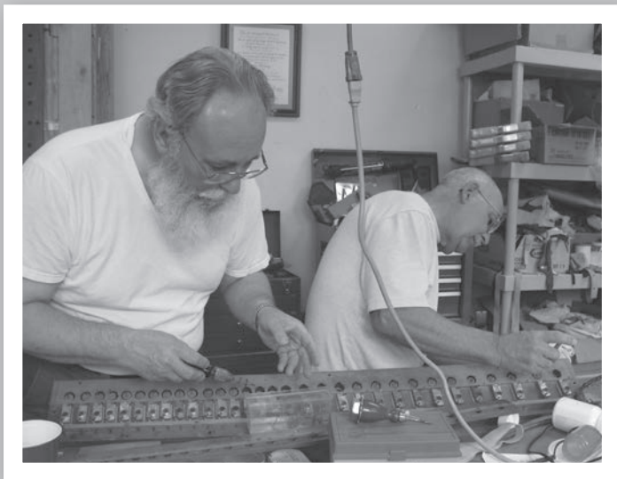
Larry and Andy Gallien install new primary valves
