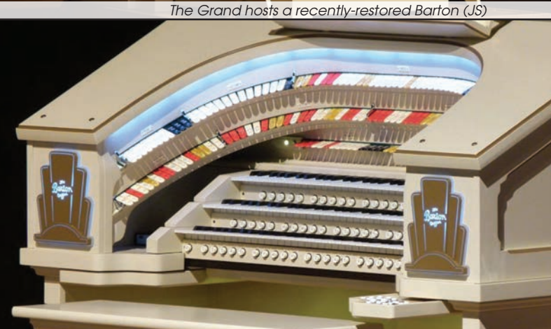
The console has been equipped with LED lighting, which also shines behind and through the front-panel nameplates (PB)
