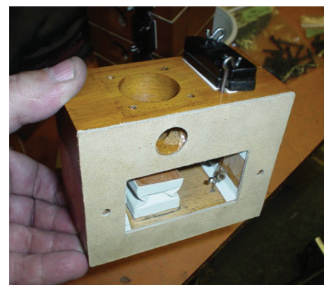
A rebuilt primary box. Notice the leather sealing strips in the interior corners
