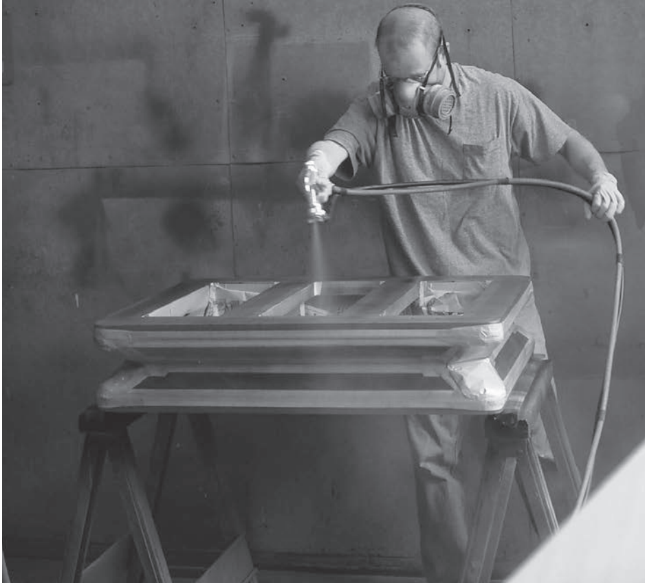
All the wood receives a new finish. Here, Justin Nimmo applies finish to a rebuilt reservoir
