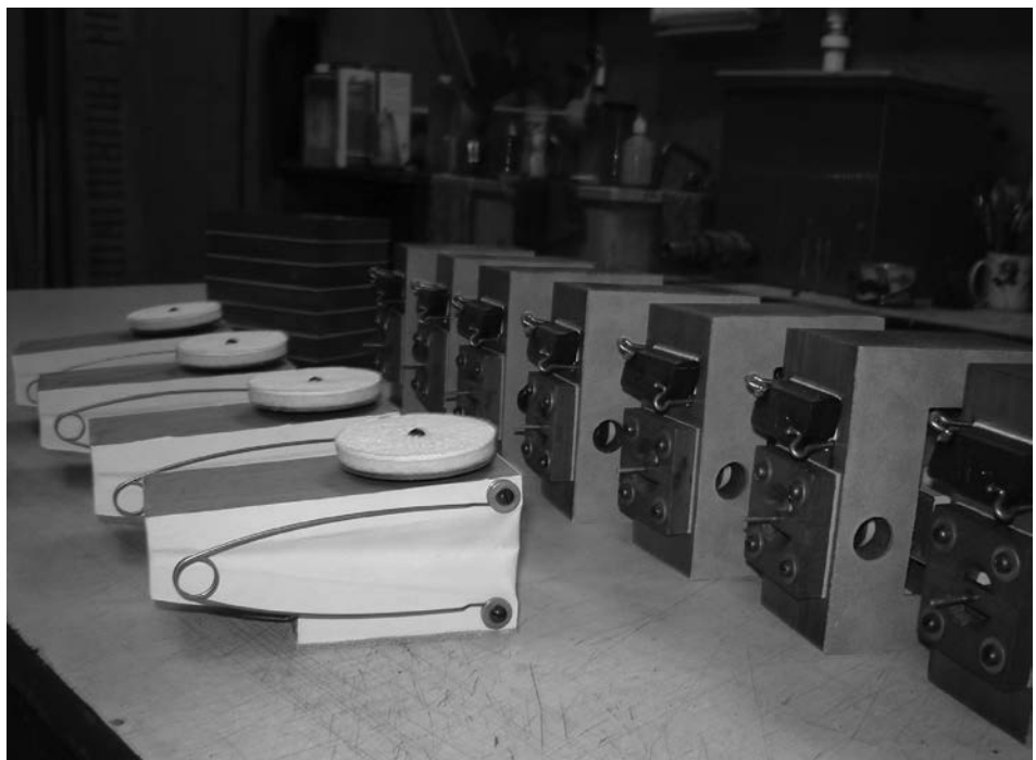
Restored pallets in the Tibia offset chest Tuba offset pneumatics and primary boxes ready for installation
