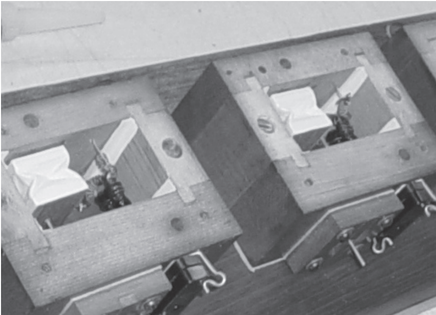
A perfectly-adjusted primary valve and pneumatic assembly. With the valve seated, the pneumatic is not fully extended. (Photo by the Carlton Smith)
