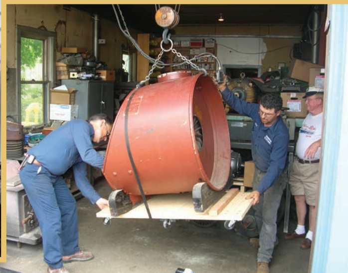
The five-horsepower blower is delivered to Manion Electric in Plattsburgh for restoration
