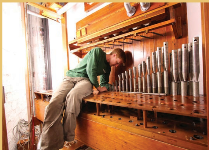
Jonathan Ortloff plants pipes of the Vox Humana in the Solo chamber (Photo by Joseph Rotella)
