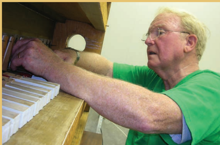
Ernie Dossin installs pallets in the Solo chest
