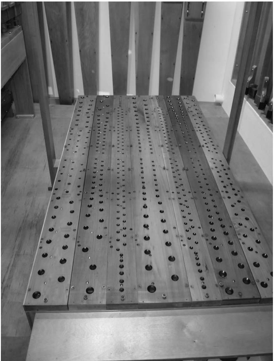
The finished manifold clamped in place during test fitting on the chest
