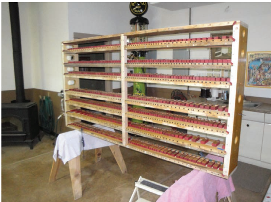
The re-cut half-lap joints were tested for fit before the newly-doweled ends were redrilled. The bottom cross brace on the original seven-rank chest was unusable, so a replica was made
