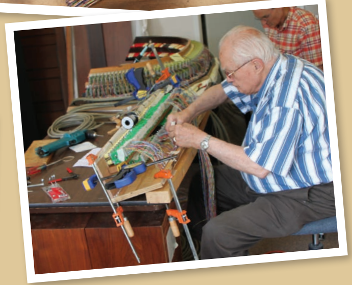
The backrail SAMS are temporarily clamped to a layout fixture to lay out the wiring harness (Photo by Clink Meadway)
