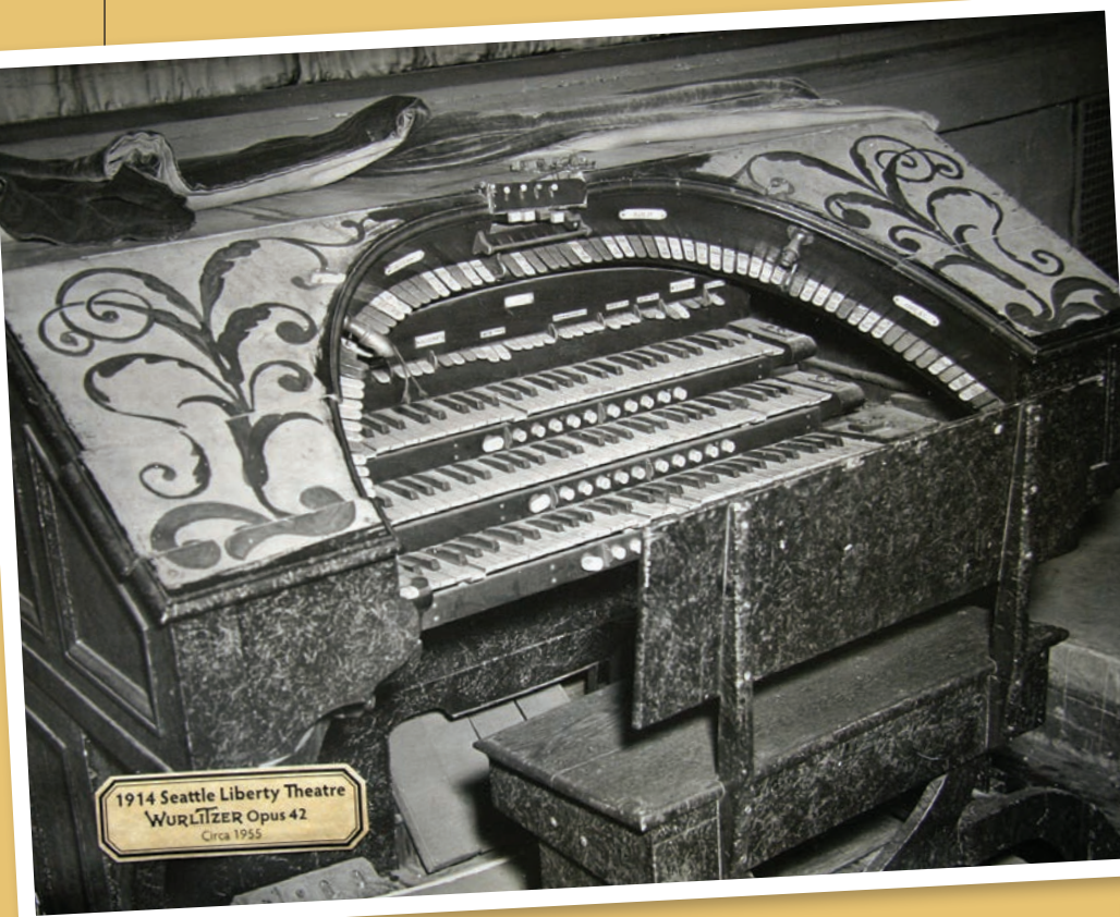
The Liberty console in the theatre, 1955. The indignities suffered by the console over the previous 40 years are apparent: note the broken lid, unique finish, keys apparently missing return springs, broken light fixtures, and missing toe studs (Bill Bunch collection)
