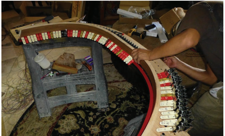
Installing SAMs. Stop keys were “glued” to SAMs with burnt shellac
