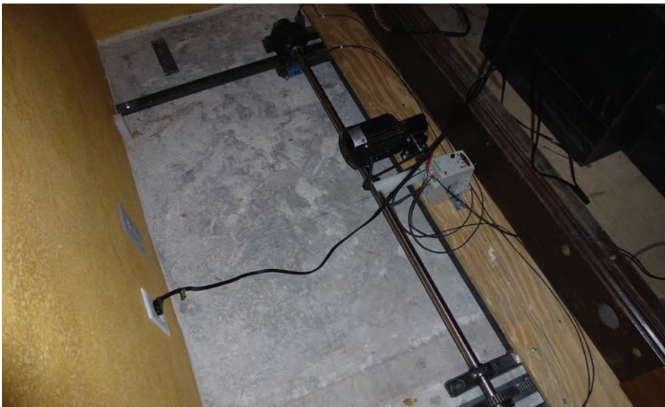
Detail of gear drive which acts as support wheels for back of platform
