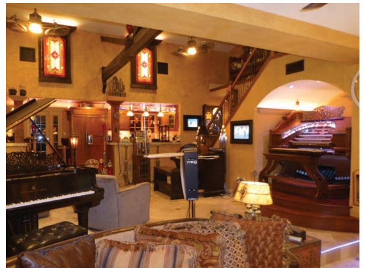
Leaded glass "windows" in upper background hide Leslie 122R speakers for the Hammond RT-3; they open pneumatically
