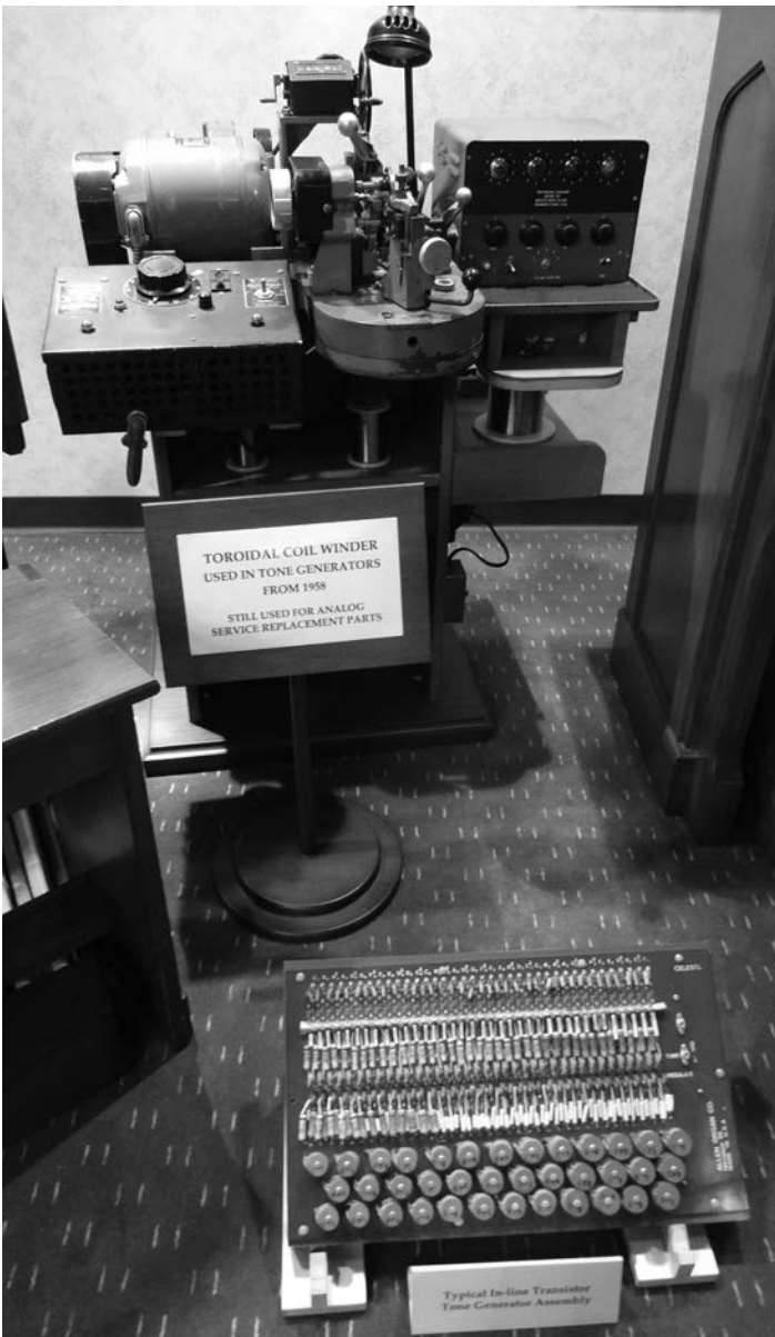
The machine at the top is a "Toroidal Coil Winder," used in analog tone generators (and still used in the manufacture of replacement parts).
