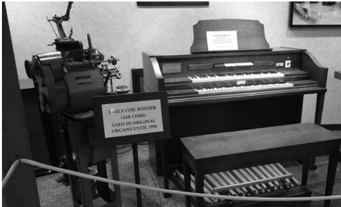
The machine on the left is a coil winder; the organ is a model S-5 from 1950, which had internal tone generators and used external speakers
