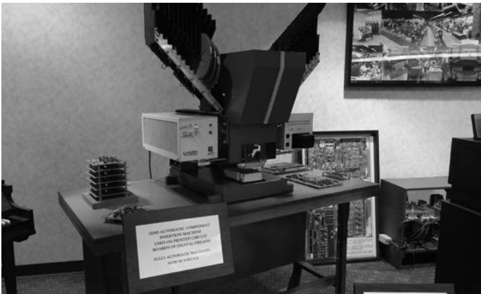
Prior to fully-automated machines being developed, semi-automatic machines such as this one were used to install components on circuit boards.
