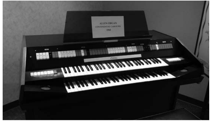
1968's Continental Carousel represented a significant advance, both in styling and capability. It contained a synthesizer and a feature called "Flying Hammers" which utilized velocity-sensitive keying to produce a "strumming" effect.
