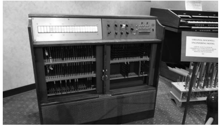
The original "Rockwell Engineering Model" from 1969, used by Allen to develop commercially viable digital organs using large scale integrated (MOS/LSI) circuit devices.
