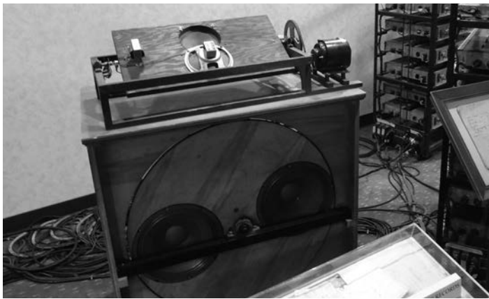
You recognize the Gyrophonic cabinet, but probably not the test jig on top. That was another experiment in "moving speaker" technology
