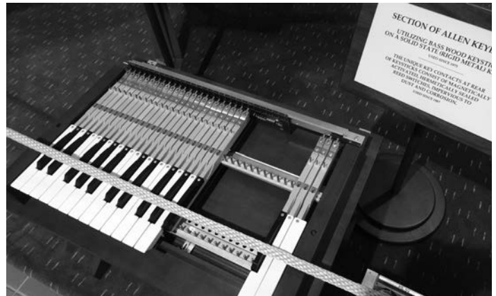
This cutaway keyboard model shows the construction and keying system used by Allen keyboards since 1987.
