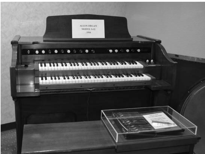
A model S-12 from 1954, using drawknobs for stops. The light-colored knobs are the even pitches, the dark knobs are mutations.
