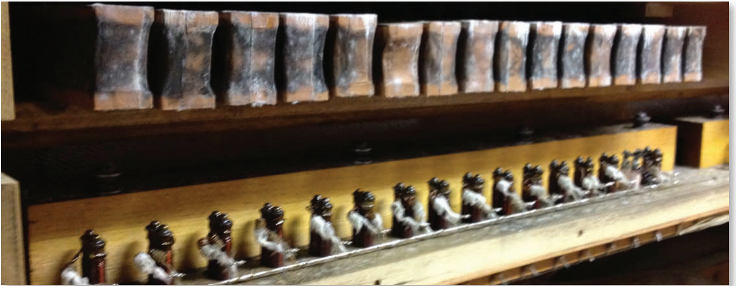
Armory Switchstack Pneumatics (Photo by Doug Powers)
