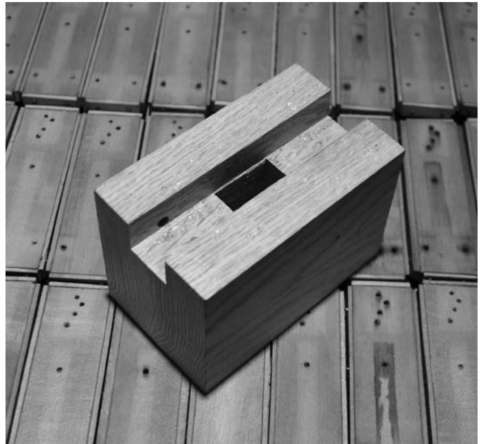
Although it appears to be made from a solid block of wood, it isn't; it's just two pieces screwed together
