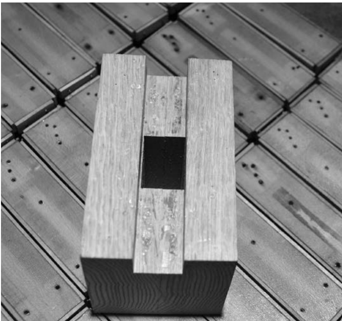
The top groove is just slightly wider than the mortise; since the pneumatic lays in it lengthwise, it doesn't need to be quite as close-fitting as the mortise, where the pneumatic stands on end
