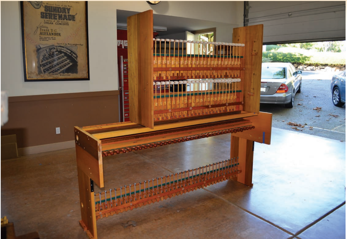
Here's the stack being fit together, without bars and resonators.
