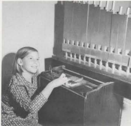
The console is built around the source of keys—a discarded toy piano. Debbie needs no drawknobs or stopkeys. Her one rank of Stopped Flutes is "on" all of the time. The tone is Tibia-like.
