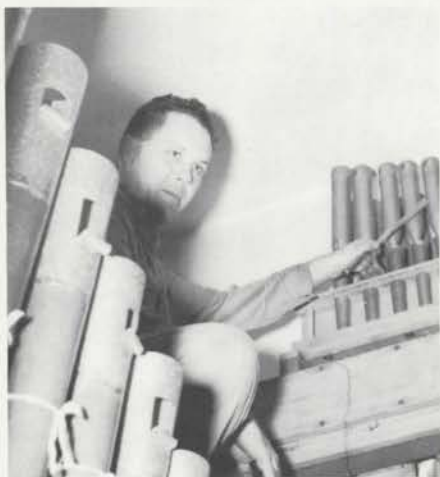
CREW CHIEF DICK STONEY listens to the just-tuned Vox Humana, which is mounted on a separate chest above the swell shutters in the Swell Chamber. Cornopean pipes are in left foreground.
