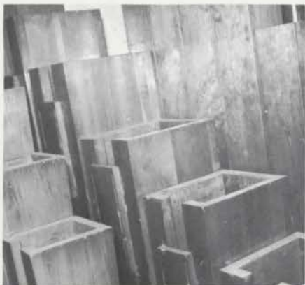
BIG GROWLERS in the Pedal Organ. L. to r.: Trombone, Double Open Diapason, Violone and Open Diapason. These huge pipes occupy considerable space in the left side of the hall. They are unenclosed. Curiously, the instrument has no Diaphone.
