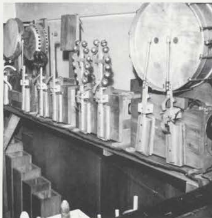
THEATRICAL EFFECTS are provided by Snare Drum, Sleigh Bells, Wood Block and many other noisemakers and percussions. A Bass Drum is out of range, and that's part of the Bourdon below. These are in the Choir Chamber.
