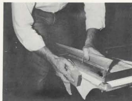
Sanding smooth side of hinge leather prior to gluing. Note finishing nails (arrow) holding fold in place and nail holding fold open.
