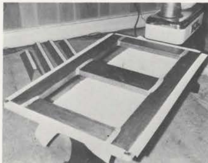
Gluing hinge strips to regulator head. Note folds in background.
