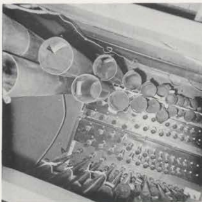
A squatty Kinura rank separates two chests of Tuba pipes.
