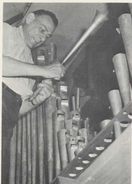
Paul Lewis, Vice Chairman and Program Chairman for CATOE, adjusts foot on a reed pipe.
