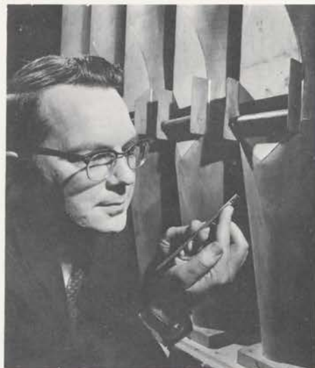
The largest and smallest pipes in the great chamber. Dr. Beaupre shows that the speaking part of the smallest is no bigger than his fingernail while the Double Diapasons are almost two feet in diameter and up to 16 feet tall.
