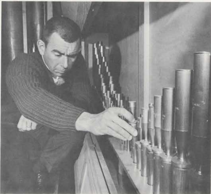
Vox Humana in the swell chamber is enclosed in a wooden resonating chamber. George Kebt, U.R.I. organist in residence, inspects a ciphering reed.
