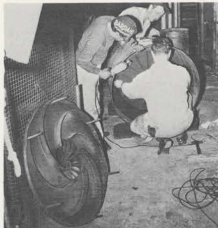
Val Escobar (standing left), Frank Pokorny (standing rear), Jack Smith pull the blower rotor at Lima.
