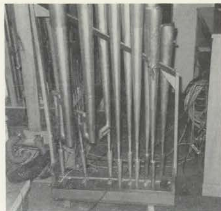
Nine-note Trumpet offset chest being tested (May, 1965).
