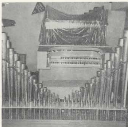
Reed chest assembled (March, 1965). Pipes are Cornopean revoiced as Trumpet. Console in background.
