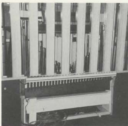
Glass swell shades are not pivoted but slide in grooves to fill spaces between wooden columns for lowest volume.
