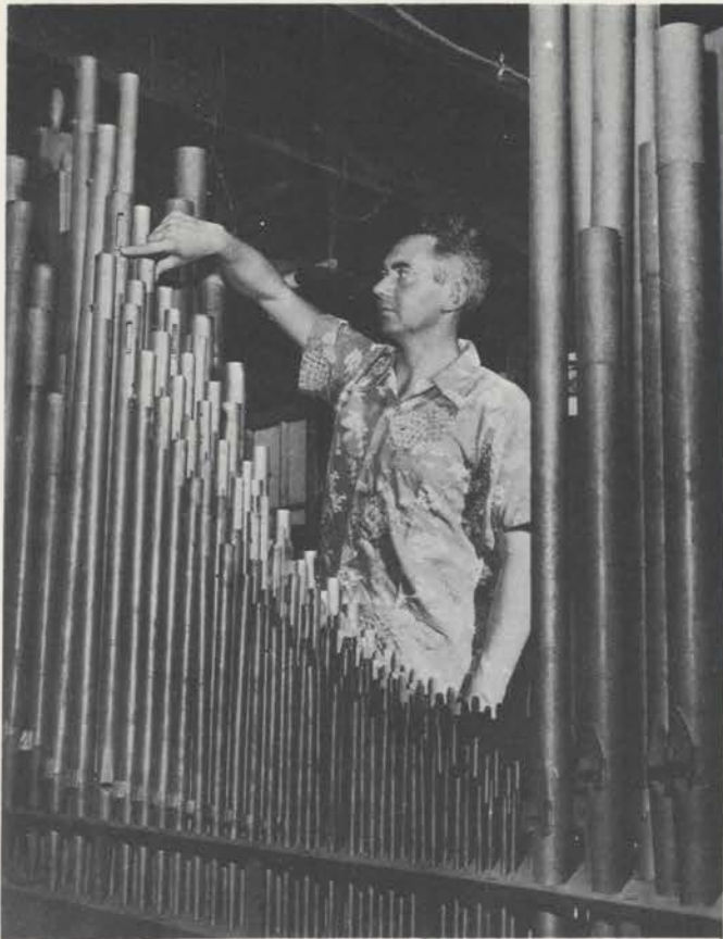
Jim adjusts a tuning roll on a string pipe.
