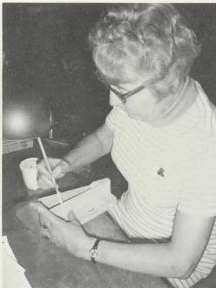
Application of Perflex is similar to leather or rubber cloth. Note glue container has plastic top with hole for brush to reduce formation of skin on top of glue.
