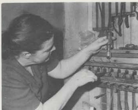
Cassie Baker adjusts valves in switchstack of relay.
