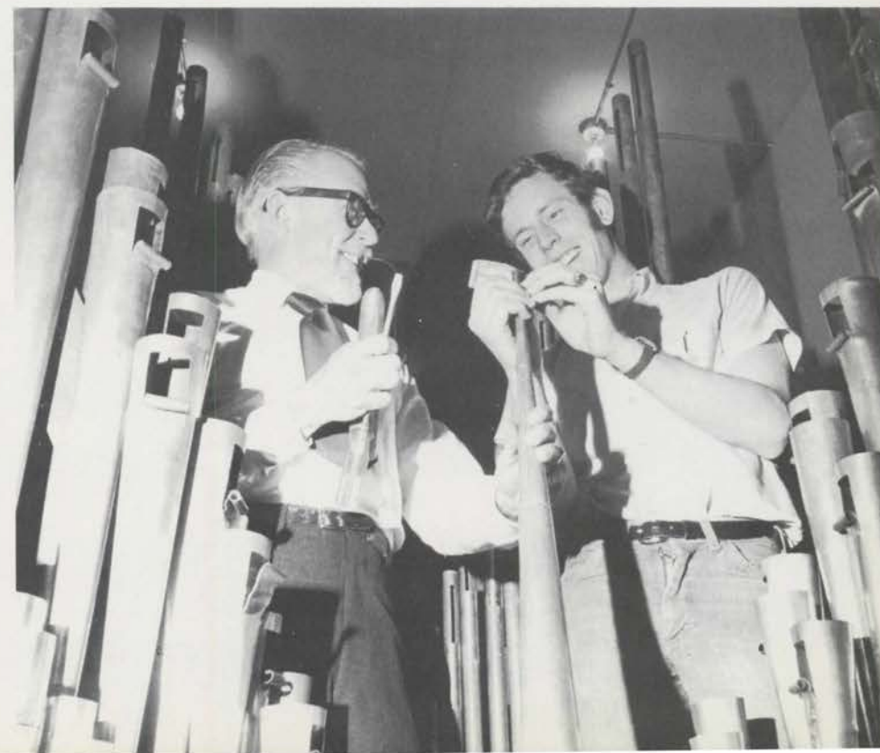
Bert Buhrman and the head of the student crew on organ maintenance, James Fisher, clean the reed of a Tuba pipe with a five-dollar bill. National currency does not leave lint when used in this fashion. — (Bert Buhrman collection)
