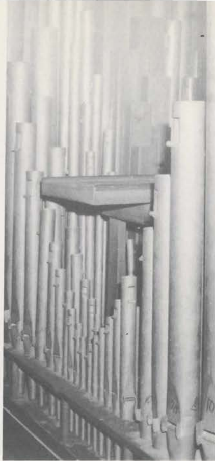
P.K. Johnson's swell chamber for Kimball. Top of chest is even with the studio floor.
