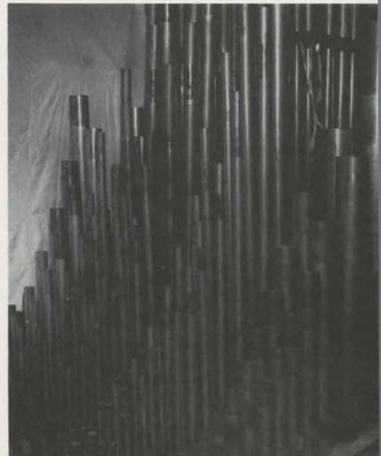
Foundation chamber showing from left: Vox Humana, Harmonic Flute, Gamba, Gamba Celeste, 10" Tibia Clausa, Solo String, and Diaphonic Diapason.
