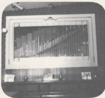
Through the shutter glass, Pipes are clearly visible through the transparent swell shutters. — (Stufoto)
