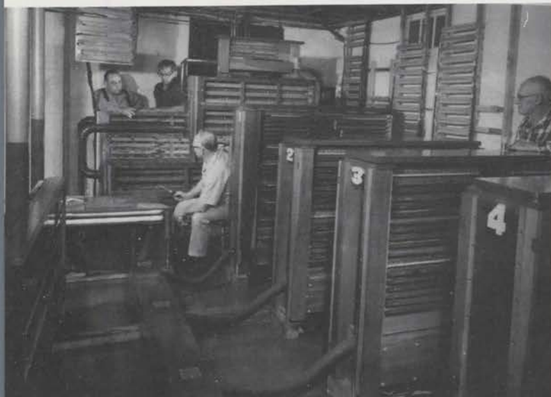
Relay room in basement was scene of hectic activity for many months. 1st and 2nd touch relays in rear, surmounted by small Tibia mutation switch (note blower starter switch). Four switch stacks at right, pizzicato relay at left. Behind camera is special relay (1st and 2nd) for fourth manual. Left to right: George Denham, Ron Oberholtzer, Bob Lent and Ed (Tonawanda) Dornfeld.
