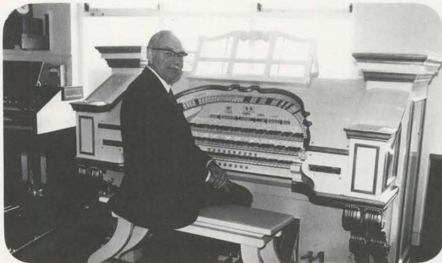
Roy Bingham at the 'M Ranch' 3/8 Wurlitzer. Note wide decorative end columns and fluted, double bolsters supporting side jambs. This is apparently a British design which marks a number of England's Wurlitzers.
