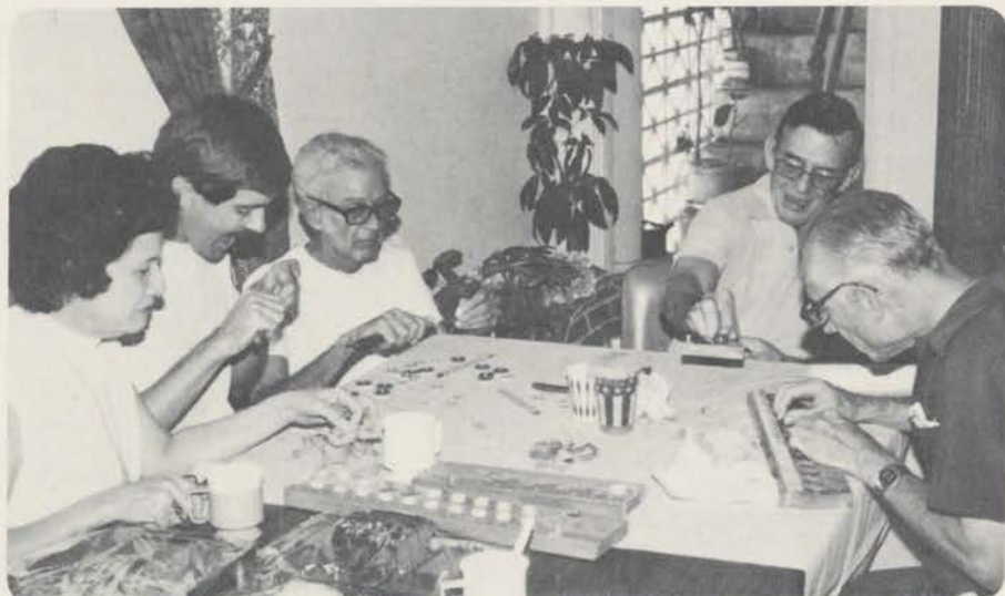
Aloha Chapter members busy at work releathering the pouch rails of the old Robert Morton organ they are trying to preserve. (L to R) Mary Chandler, Scott Bosch, Frank Loney, Jim Chandler and Bob Anderson.
