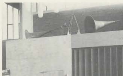
Melotone electrostatic unit is visible atop the chambers of the 3/16 Compton at St. John Vianney Church, Clayhall.
