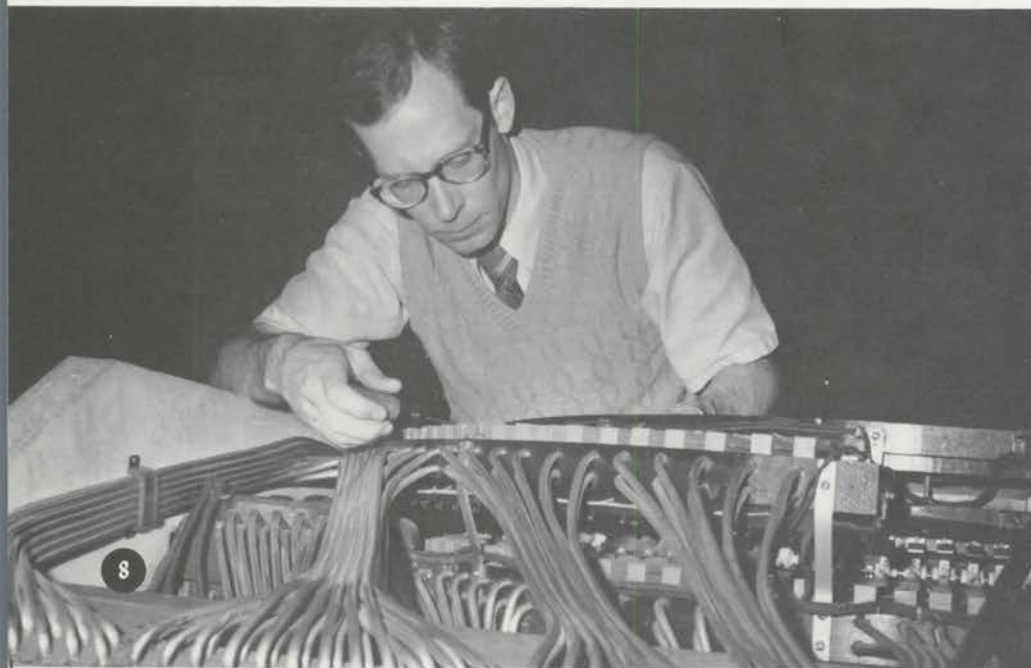
Dick Taylor adjusts a stop tab spring in the console. Note original combination action.
