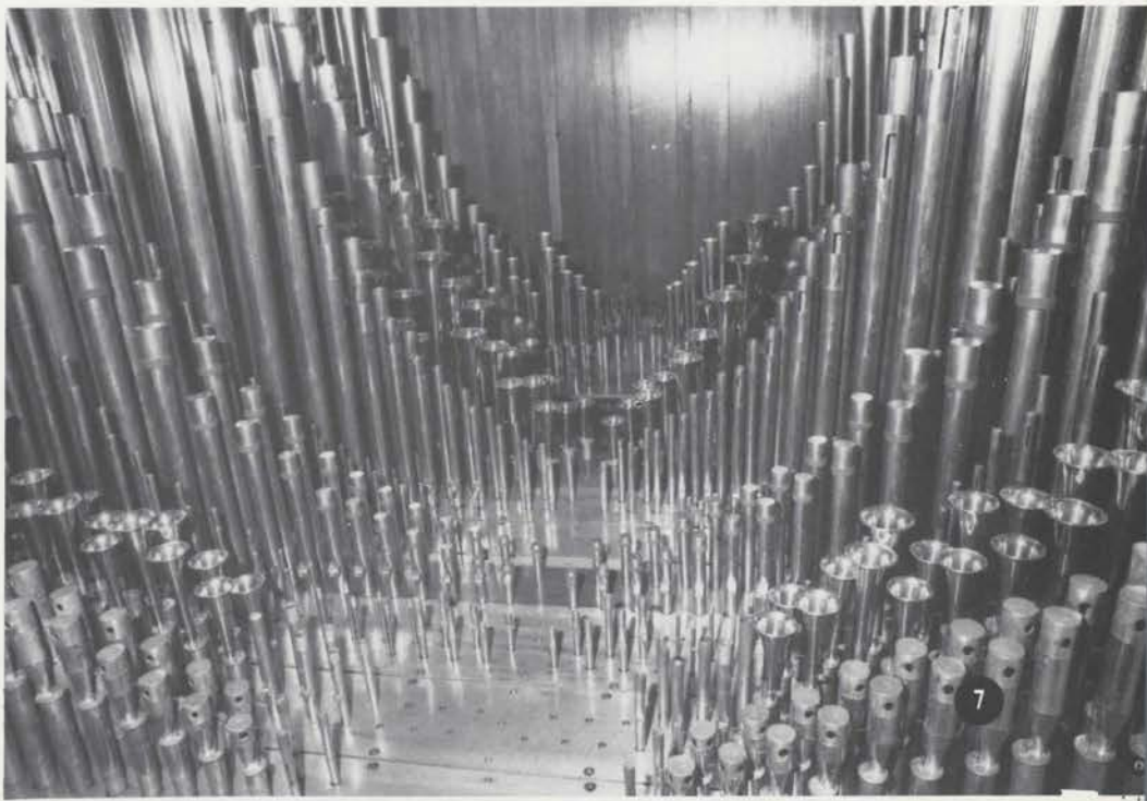
Solo Chamber showing from front to back: Vox Humana, Brass Saxophone, Gamba, Quintadena, Gamba Celeste, Horn Diapason, Brass Trumpet, Tuba Mirabilis and English Horn. Partially visible behind English Horn are the Solo Tibia Clausa, Orchestral Oboe and Kinura.
