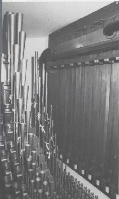
Front chest in Solo Chamber showing left to right: Tuba Mirabilis, English Horn, Solo Tibia Clausa, Orchestral Oboe and Kinura.
