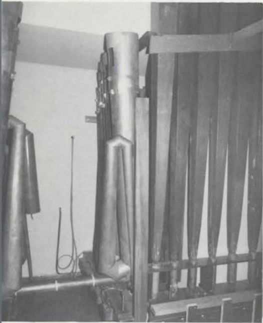
Main chamber. Metal pipes are rare 16' Wurlitzer Diaphone (on 15" wind); wood pipes are Morton 16' Tuba.
